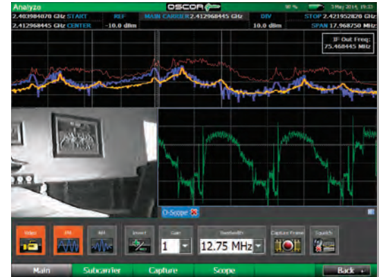
Demodulated video signal in Analyze mode
