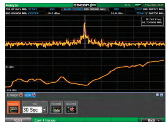
Demodulated audio signal in Analyze mode
